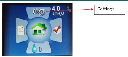
Enter the Settings screen by pushing the Up button to highlight the icon, then press the Center button to select it.
