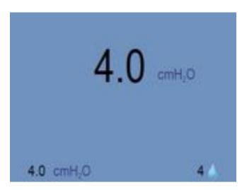
The blue droplet indicates that the humidifier is active. Note: This includes cases where decreased water quality (tap water) was detected.
