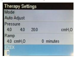
Push the Up or Down button to move the value from 0 to 3. A setting of 0 provides no exhalation relief, 3 provides the greatest exhalation relief. Press the Center button to save your selection.
