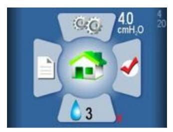
Indicated by a flashing red X. The humidifier will be disabled. Caused by:
