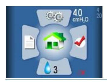
Indicated by a flashing red droplet and red 'X'. The humidifier will be disabled during therapy.
