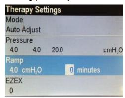
Use the Right button to highlight and the Center button to select Ramp Duration in minutes. Press the Up or Down buttons to change the duration from 0 to 45 minutes, moving through increments of five minutes. **Press the Center button to save your selection.**
