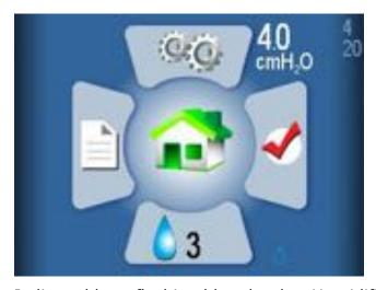
Indicated by a flashing blue droplet. Humidifier will be disabled during therapy. Can be caused by:
