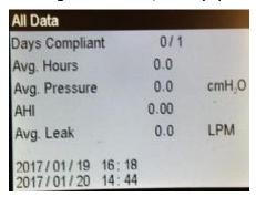
In All Data you will see data for all the days you've been using the device. This screen shows a time stamp in the bottom left of how long the device has been in use.
