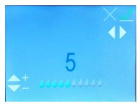
Use the Up or Down buttons to move the humidification level from 0 to 10 (0 = no humidification, 10 = maximum humidification). You will see the water droplet icons move to a higher or lower value. Once you reach the desired setting, use the Left and Right buttons to toggle to the green checkmark, if it's not already highlighted, then press the Center button to save your settings.
