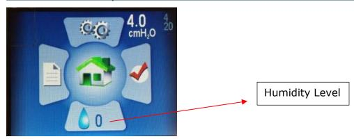
From the Home screen, push the Down button to highlight the Humidifier section. Push the Center button to select it.
